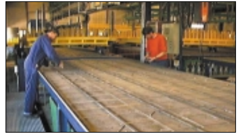
▲ Precision location of parts on working tables.
