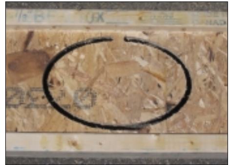
▲ With the VIP System's add-on router unit, service holes can be cut into engineered wood I-joists at the same time as the cross-cutting.
