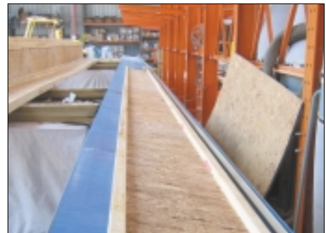
▲ The Virtek I-Joist Processing System processes up to 2,500 linear feet every hour, handling lengths of up to 60 feet.
