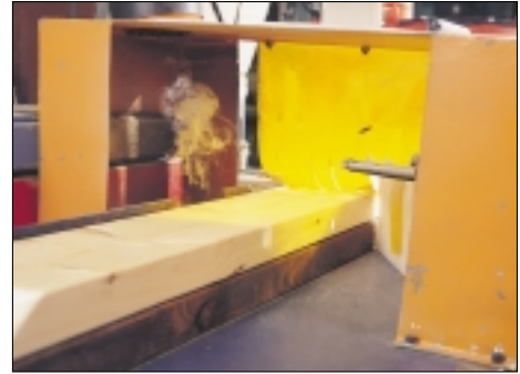
▲ LaserMC automatically moves the lumber into position, where it is marked for each joint location.
